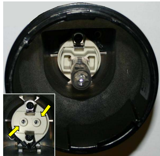
Figure 2. Opened lamp housing. Lamp holder (inset L). Pull the old lamp out by its base to remove it. Insert the new lamp and push it in until it is fully seated.
