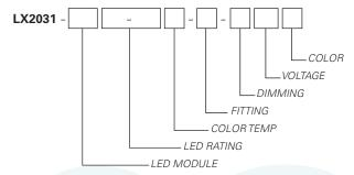
Example Part Number: **LX2031-T1910-9830-0E-TE120W** is a fixture with a Xicato 19mm LED module, 1050 Lumen/98 CRI/14 Watt LED rating, 3000°K Color Temperature, 0E Track fitting with Trailing Edge group dimming capability, 120V and a White finish.
