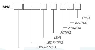
Example Part Number: **BPM-C0615-9030W-CT3-DX120W** is a fixture with a COB LED module, 1500 Lumen/90 CRI/ 3000°K Color Temperature/19 Watt LED rating, Wide Angle Lens Assembly, CT3 CONTROLTrack fitting with DMX Address knobs and DMX compatible control gear, 120V and a Black finish.
