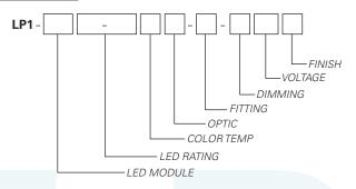
Example Part Number: **LP1-ZE410-903004-CT3-DX120W** is a fixture with a 4 LED Array module, 1090 Lumen/90 CRI/17 Watt LED rating, 3000°K Color Temperature, 35mm 4° Optic, CT3 CONTROLTrack fitting with DMX Address knobs and DMX compatible control gear, 120V and a White finish.
