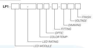
Example Part Number: **LP1-ZE410-903004-00-TE120W** is a fixture with a 4 LED Array module, 1090 Lumen/90 CRI/17 Watt LED rating, 3000°K Color Temperature, 35mm 4° Optic, 00 Track fitting with Trailing Edge group dimming capability, 120V and a White finish.
