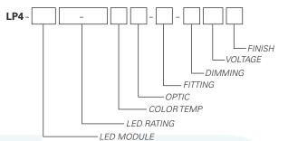
Example Part Number: **LP4-C1965-903510-00-TE120W** is a fixture with a high power, 19mm COB LED, 6500 Lumen/90 CRI/78 Watt LED rating, 3500K Color Temperature, 180mm 10° Optic, 00 Track fitting with Trailing Edge group dimming capability, 120V and a White finish.
