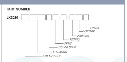
Example Part Number: **LX2020-ZE102-903004-CT4-DX120W** is a fixture with a single LED module, 270 Lumen/90 CRI/4 Watt LED rating, 3000°K Color Temperature, 35mm 4° Optic, CT4 CONTROLTrack fitting with DMX Address knobs and DMX compatible control gear, 120V and a White finish.
