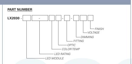
Example Part Number: **LX2030-ZE102-903004-CT4-DX120W** is a fixture with a single COB LED module, 270 Lumen/90 CRI/4 Watt LED rating, 3000° Color Temperature, 35mm 4° Optic, CT4 CONTROLTrack fitting with DMX compatible control gear, 120V and a White finish.
