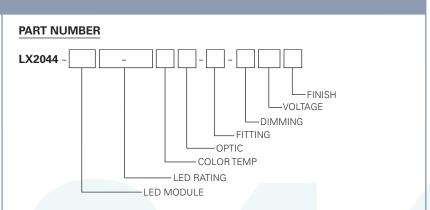
Example Part Number: **LX2044-B1820-92TWW2-PT5-ED120W** is a fixture with a Tunable White LED module, 2000 Lumen/92 CRI/22 Watt LED rating, Tunable White 2700K-6500K Color Temperature, 72mm 20° Optic, PT5 Track fitting with Integral Dimming/CCT setting capability, 120V and a White finish
