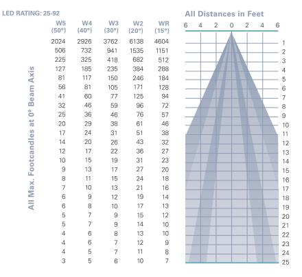
Photometric Data based on LED Rating: 20-92 (2000 Lumens/92CRI/22watts)
