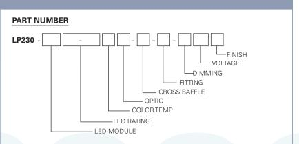
Example Part Number: **LP230-ZE308-903004-NXB-CT4-DX-120W** is a fixture with a ZE3 LED module, 810 Lumen/90 CRI/13 Watt LED rating, 3000°K Color Temperature, 4° Optic, No Cross Baffle, CT4 CONTROLTrack fitting with DMX Address knobs and DMX compatible control gear, 120V and a White finish.
