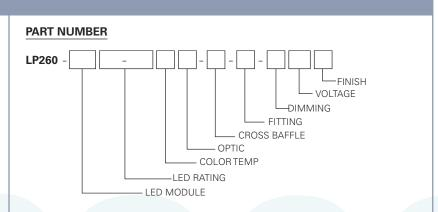
Example Part Number: **LP260-ZE102-903004-NXB-CT4-DX120W** is a fixture with a single COB LED module, 270 Lumen/90 CRI/4 Watt LED rating, 3000° Color Temperature, 35mm 4° Optic, No Cross Baffle, CT4 CONTROLTrack fitting with DMX compatible control gear, 120V and a White finish.
