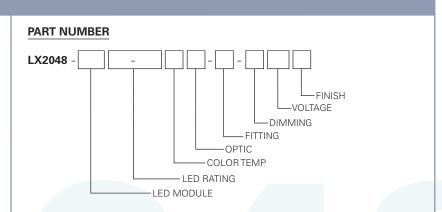
Example Part Number: **LX2048-B1820-92TWW2-CT3-DX120W** is a fixture with a Tunable White LED module, 2000 Lumen/92 CRI/22 Watt LED rating, Tunable White 2700K-6500K Color Temperature, 72mm 20° Optic, CT3 CONTROLTrack fitting with DMX Address knobs and DMX compatible control gear, 120V and a White finish.
