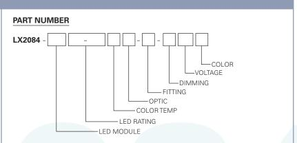
Example Part Number: **LX2084-V1861-9030K1-CT3-DX120W** is a fixture with a Bridgelux 18mm LED module, 6100 Lumen/90 CRI/58 Watt LED rating, 3000K Color Temperature, 111mm 10° Optic, CT3 CONTROLTrack fitting with DMX Address knobs and DMX compatible control gear, 120V and a White finish.
