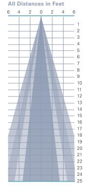
Photometric Data based on LED Rating: 61-90 (6100 Lumens/90CRI/58watts)
