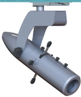
The miniature BPM series is a professional grade high output LED instrument with features such as 360 degree gate rotation, true "E" size gobo projection, 3 plane cool touch shutters and easily changed zoom lenses (narrow and wide).
