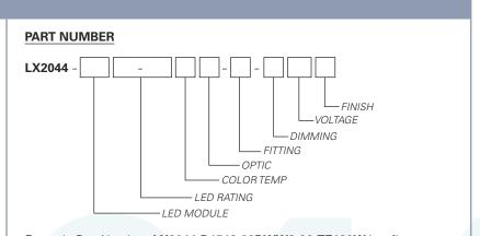
Example Part Number: **LX2044-D1518-92DWW2-00-TE120W** is a fixture with a Dim to Warm LED module, 1800 Lumen/92 CRI/22 Watt LED rating, 2800° - 2000°K Color Temperature, 72mm 20° Color Mixing Optic, 00 Track fitting with Trailing Edge group dimming capability, 120V and a White finish.
