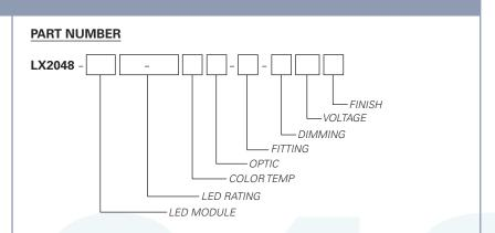
Example Part Number: LX2048-D1518-92DWW2-CT1-10120W is a fixture with a Dim to Warm LED module, 1800 Lumen/92 CRI/22 Watt LED rating, 2800° - 2000°K Color Temperature, 72mm 20° Color Mixing Optic, CT1 CONTROLTrack fitting with 0-10V compatible control gear, 120V and a White finish.
