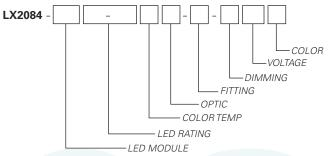
Example Part Number: **LX2084-T1930-9830K1-CT3-DX120W** is a fixture with a Xicato 19mm LED module, 3000 Lumen/98 CRI/41 Watt LED rating, 3000K Color Temperature, 111mm 10° Optic, CT3 CONTROLTrack fitting with DMX Address knobs and DMX compatible control gear, 120V and a White finish.
