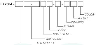
Example Part Number: **LX2084-D1530-92DWW2-00-TE120W** is a fixture with a Dim to Warm LED module, 3000 Lumen/92 CRI/44 Watt LED rating, 3000-2000K Color Temperature, 72mm 20° Color Mixing Optic, 00 Track fitting with Trailing Edge group dimming capability, 120V and a White finish.
