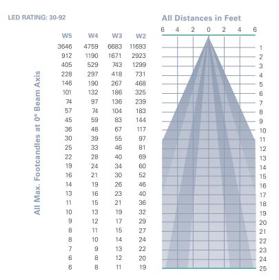
Photometric Data based on LED Rating: 30-92 (3000 Lumens/92CRI/42watts)
