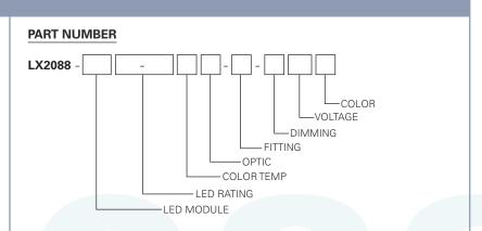
Example Part Number: **LX2088-B1841-92TWW2-CT3-DX120W** is a fixture with a Tunable White 18mm LED module, 4100 Lumen/92 CRI/52 Watt LED rating, Tunable White 2700K-6500K Color Temperature, 72mm 20° Optic, CT3 CONTROLTrack fitting with DMX Address knobs and DMX compatible control gear, 120V and a White finish.
