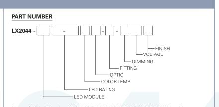
Example Part Number: **LX2044-V1828-9030M2-CT3-DX120W** is a fixture with a Bridgelux 18mm LED module, 2800 Lumen/90 CRI/23 Watt LED rating, 3000°K Color Temperature, 70mm 20° Optic, CT3 CONTROLTrack fitting with DMX Address knobs and DMX compatible control gear, 120V and a White finish.
