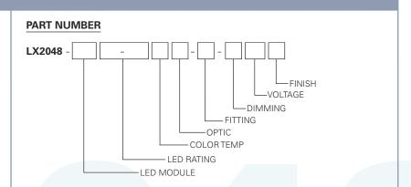
Example Part Number: **LX2044-V1828-9030M2-CT3-DX120W** is a fixture with a Bridgelux 18mm LED module, 2800 Lumen/90 CRI/23 Watt LED rating, 3000°K Color Temperature, 70mm 20° Optic, CT3 CONTROLTrack fitting with DMX Address knobs and DMX compatible control gear, 120V and a White finish.
