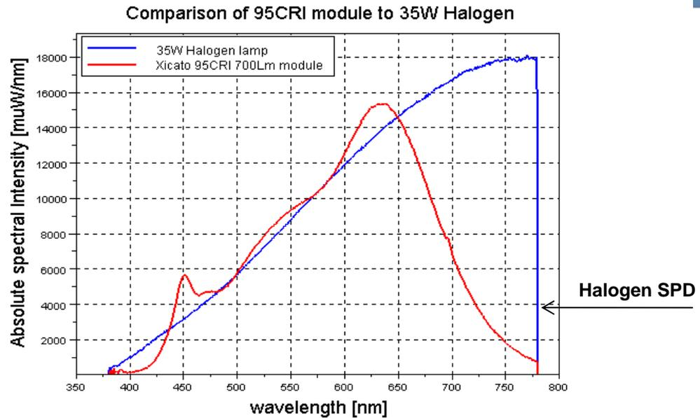
2. CRI: The Color Rendering Index (CRI) of a halogen lamp is near 100, meaning that it will render all artwork well. In theory, a source with an incandescent filament (which is what a halogen lamp is) creates full spectrum light with a CRI close to 100. In practice, the coatings that are typically used in today's halogen lamps introduce small shifts in spectrum that sometimes causes a halogen lamp to exhibit a CRI with a value less than 100, say 97 or 98.
