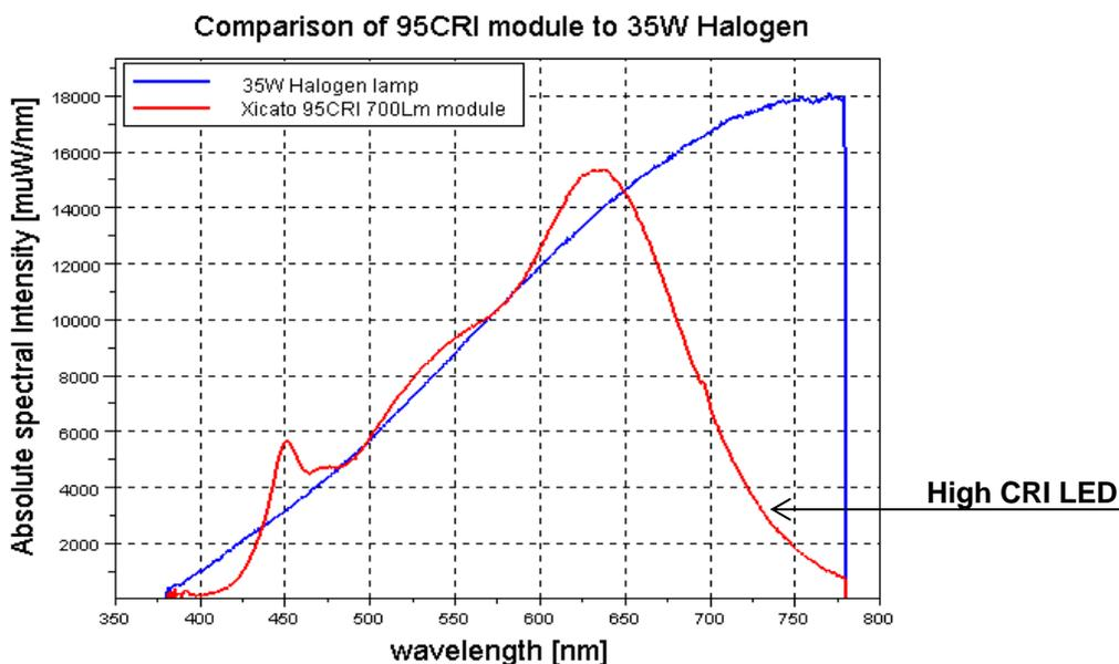
2. **CRI:** The color rendering index of this source is as high as 98CRI, using the current metric. This has been verified by several independent testing laboratories, using the same metrics that would typically be used to measure a halogen, or any other source. This CRI, when compared to a halogen source is virtually identical, and in fact measures higher in some areas such as R9 (deep red).
