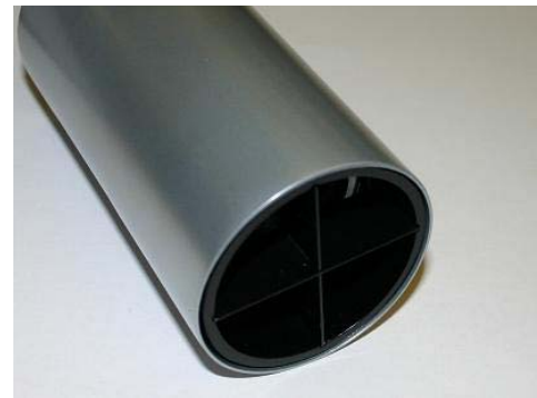
Figure 9. Remove Cross-Baffle cartridge assembly by pulling it out of the cylinder housing. Cross-Baffle should be flush or below front edge of housing when installed.
