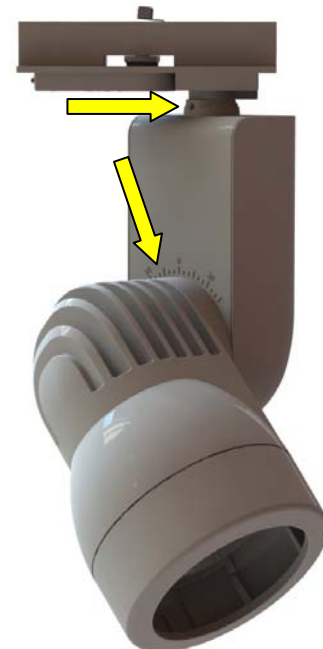
Figure 12. Horizontal focus lock (top arrow). Vertical focus lock (bottom arrow).
