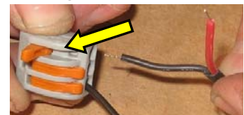
Figure 16. A Quick Connector with tab lifted. Ensure that one connector has two black wires and the other connector has a red wire and a purple wire.
