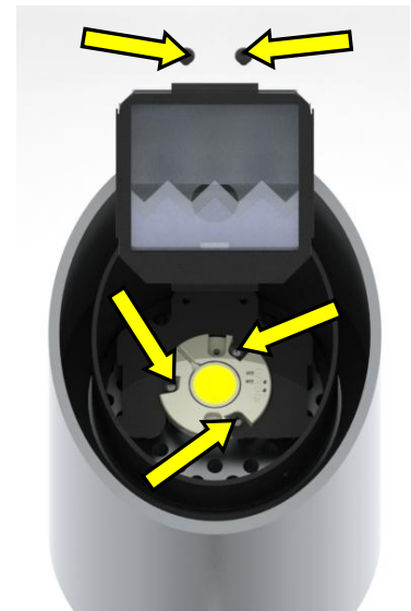
Figure 12. Remove the reflector assembly by removing the two assembly screws, and then remove the 3 screws holding the LED.
