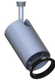
Figure 6. Remove Cross-Baffle cartridge assembly by pulling it out of the cylinder housing. Cross-Baffle should be flush or below front edge of housing when installed.
