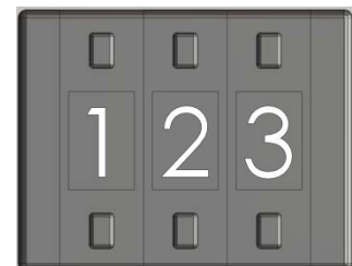
Figure 22. DMX address, 3 digit push button
