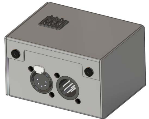
Figure 20. DMX controller housing
